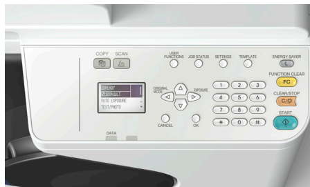
e-STUDIO2802AM Control Panel
